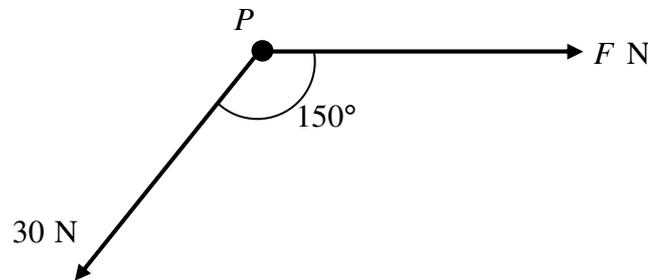
Two forces, act on a particle  $P$  so that the angle between the two forces is  $150^\circ$ .
