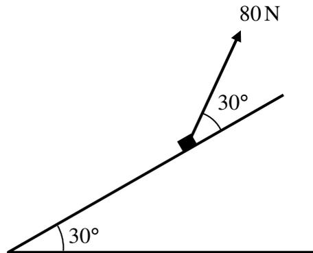
A box of mass 10 kg is pulled by a rope on a fixed rough inclined plane. The rope is modelled as a light inextensible string and the box is modelled as a particle. The plane is at an angle of  $30^\circ$  to the horizontal, as shown in the figure above.
