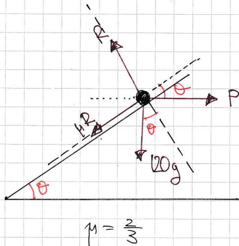
RESOLVING PARALLEL & PERPENDICULAR TO THE PLANE
