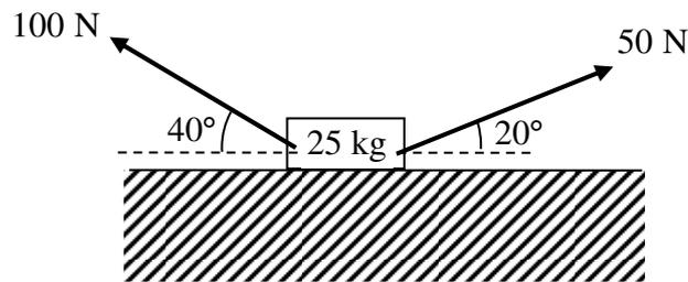
The figure above shows a small box of mass 25 kg, pulled by two light inextensible strings along rough horizontal ground.
