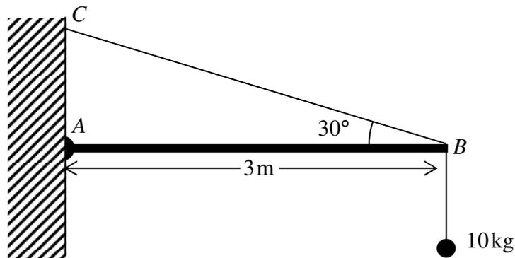
The figure above shows a uniform rod  $AB$ , of length 3 metres and of mass 20 kg, smoothly hinged at the point  $A$ , which lies on a vertical wall.
