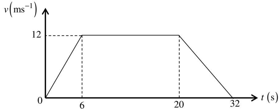
The figure above shows the speed time graph  $(t, v)$  of a car travelling along a straight horizontal road between two sets of traffic lights.
