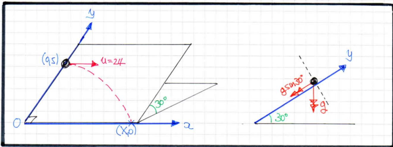
EQUATIONS OF MOTION IN  $x$  &  $y$  CAN BE SIMPLIFIED, AS THE ACCELERATION IS ZERO IN  $x$  &  $-g \sin 30^\circ$  IN  $y$
