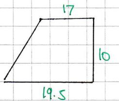
$$\begin{aligned} \text{DISTANCE} &= \frac{17+19.5}{2} \times 10 \\ &= 18.25 \times 10 \\ &= 182.5 \text{ m} \end{aligned}$$
