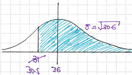
$$\begin{aligned} P(Y > 30) &= P(Y \geq 31) \\ &= P(W > 30.5) \\ &= P\left(Z > \frac{30.5 - 36}{\sqrt{30.6}}\right) \\ &= \Phi(-0.9943) \\ &= 0.8394 \end{aligned}$$
