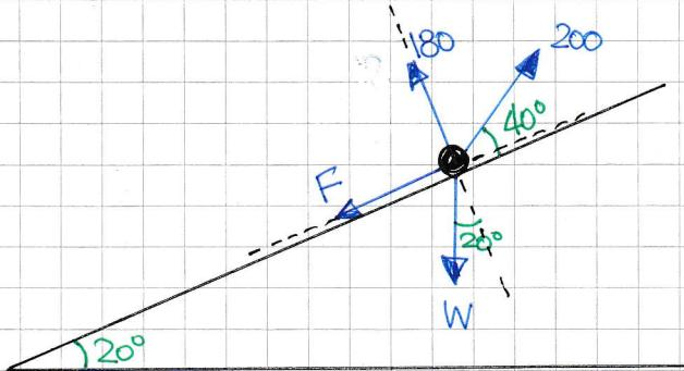
RESOLVING PARALLEL & PERPENDICULAR TO THE INCLINE PLANE
