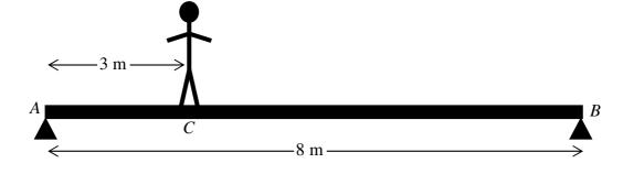
A non uniform plank of wood AB has length 8 m and mass 100 kg.
