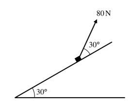
A box of mass 10 kg is pulled by a rope on a fixed rough inclined plane. The rope is modelled as a light inextensible string and the box is modelled as a particle. The plane is at an angle of 30° to the horizontal, as shown in the figure above.
