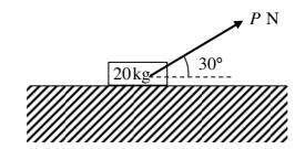
The figure above shows a small box of mass 20 kg, pulled along rough horizontal ground by a light inextensible rope, which is inclined at 30° to the horizontal.
