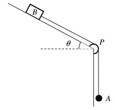
A particle A and a small box B, with respective masses of 3 kg and 7 kg, are attached to the ends of a light inextensible string.
