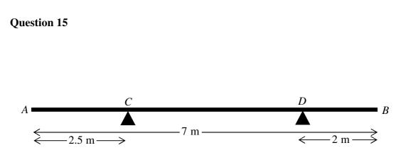
A non uniform rod AB has length 7 m and weight 300 N. The centre of mass of the rod is x m from A.
