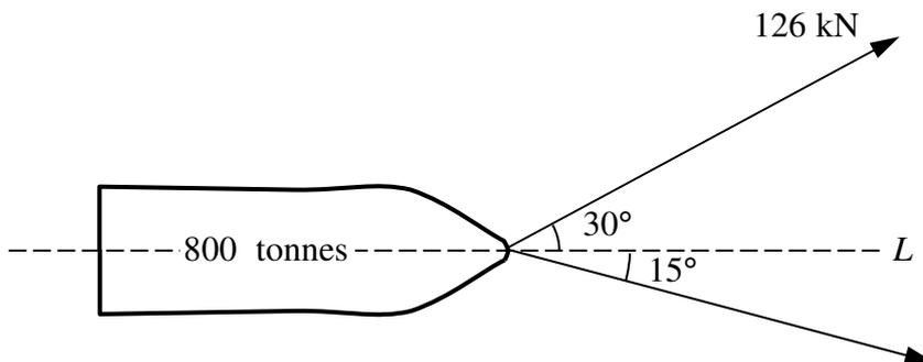
The figure above shows a ship, of mass 800 tonnes, being pulled by two tugs using horizontal cables, so that the ship is moving in a straight line  $L$ .
