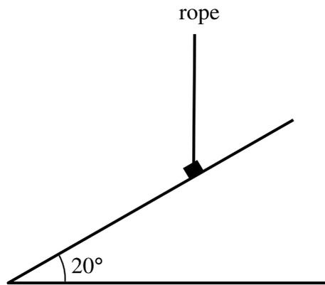
A box of mass 40 kg is held by a rope on a fixed rough inclined plane. The plane is at an angle of  $20^\circ$  to the horizontal. The rope is vertical and lies in a vertical plane containing a line of greatest slope of the incline plane, as shown in the figure above.
