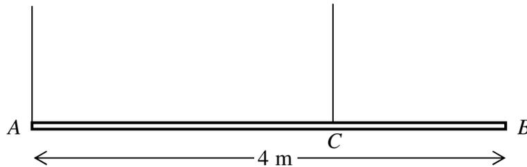
A rod  $AB$  has mass  $m$  kg and length 4 m.
